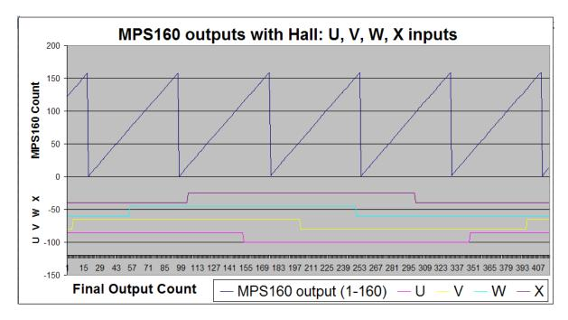
3) Use two MPS160 chips with two magnet tracks having N and N+1 poles. For this technique two MPS160 encoder ASICs are used. Each one is positioned to read one of two tracks on a rotating or linear magnet. One is magnetized with a number of magnetic poles N. The magnet on the other track is magnetized with N+1 poles (high resolution track). Each
